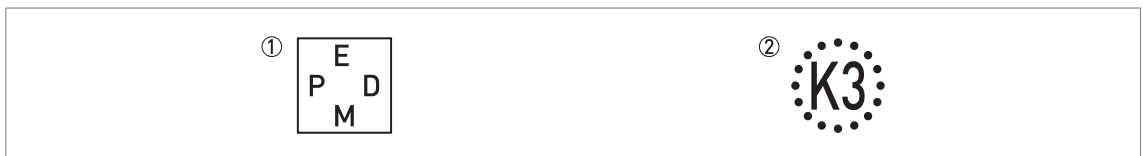
Figure 2-4: Symbols for the supplied gasket material (on the side of the process connection)
