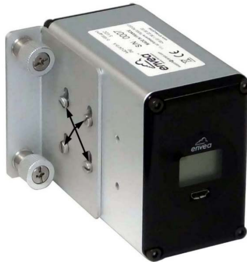
Figure 2–5 – Screwing the angle bracket on the CAIRSENS
