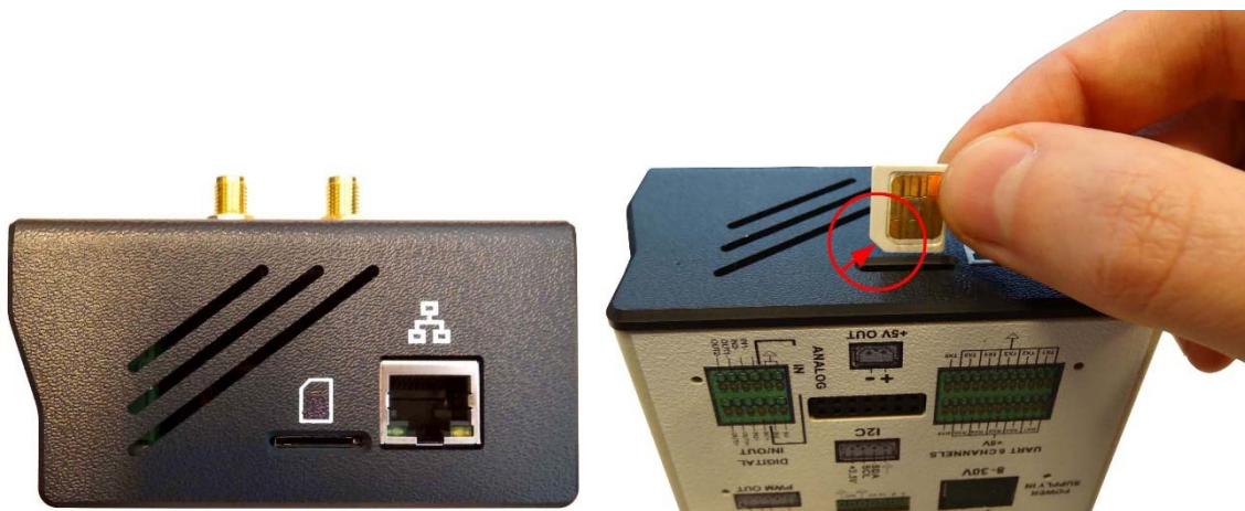
Figure 2–9 – Micro SIM card insertion
