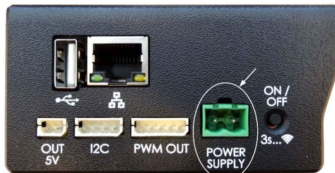
Figure 2–12 – Connection of the 2-pin connector to the 8-30 VDC IQ-LINK input
