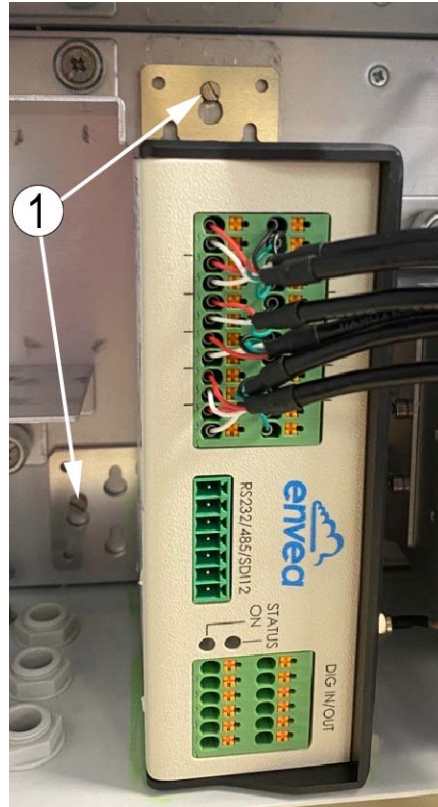
Figure 2-4 – IQ-LINK mounting bracket screws
